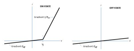
The GTO turns on if the gate-cathode voltage exceeds the specified gate trigger voltage. The device turns off if the gate-cathode voltage falls below the specified gate turn-off voltage value, or if the load current falls below the specified holding-current value.
