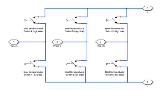
You control the gate ports of the six switching devices via an input to the Converter block G port. To do this:
