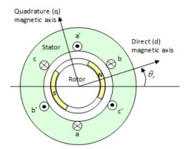
For the axes convention in the preceding figure, the a-phase and permanent magnet fluxes are aligned when rotor angle  $\theta_r$  is zero. The block supports a second rotor axis definition in which rotor angle is defined as the angle between the a-phase magnetic axis and the rotor q axis.
