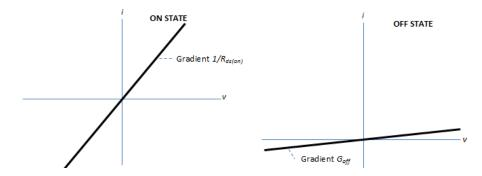
The MOSFET is in the on state if the gate-source voltage exceeds the specified threshold voltage. Otherwise the device is in the off state.
