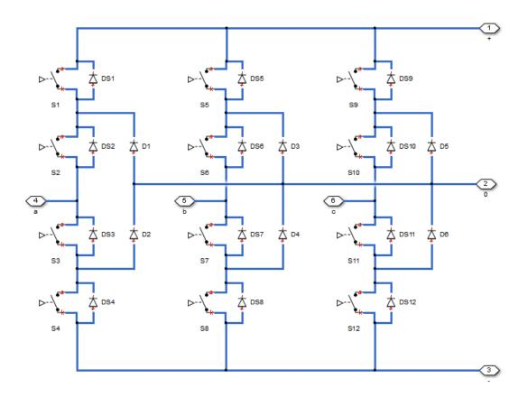
You control the gate ports of the 12 switching devices via an input to the Three-Level Converter block G port.
