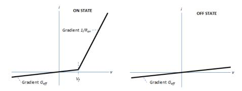
The thyristor turns on if the gate-cathode voltage exceeds the specified gate trigger voltage. The device turns off if the load current falls below the specified holding-current value.
