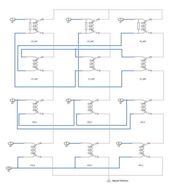
•  $W1_{zz1}$  is the primary winding located on the first limb of the core, connected between the a-phase and the negative terminal of winding  $W1_{zz5}$ .
