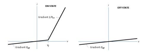
The IGBT is in the on state if the gate-emitter voltage exceeds the specified threshold voltage  $V_{th}$ . Otherwise, the device is in the off state.
